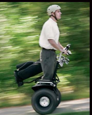
Segway Smart Motion™ technology consists of an intelligent network of sensors, mechanical assemblies, and control systems that enable the Segway PT to balance and move on two wheels. The second you step on, five micro-machined gyroscopes and two accelerometers sense the changing terrain and your body position at 100 times per second – faster than your brain can think.
